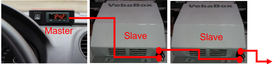
Connecting in series with remote control as master device
